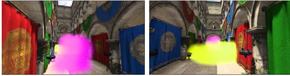
Figure 6. Two differently-colored smoke puffs in Sponza, viewed from different directions. Depth weighting by w(z, \alpha) = \alpha^2 z^{-6} gives the correct occlusion cue.
